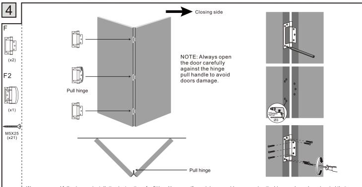
We recommend following our installation instructions for fitting. However, if your joiner considers recessing the hinges, please keep in mind that even though the hinges are 4mm, the recess cannot exceed 2mm.
