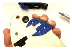
1. Hold the finderscope base against the side of the Nyx Tracker top piece as shown. Make sure it sits flush against the side, with no space visible on either side.
