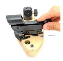
3. Slide the finderscope into the base until it snaps into place.
