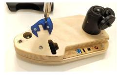
Screw the base onto the top piece of the Nyx Tracker using the three #4 wood screws. Some force will be required when starting the threads. STOP turning the screws when the base is flush against the top of the tracker. Overtightening may damage the plastic.
