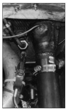
Hose clamps hold cyl # 1 slip joint onto the Anti-Reversion cone at the exhaust flange. Stainless steel 1/8" tube is silver soldered to be flush with the inner wall of the cone and provides a pressure signal to the probe/transducer.
