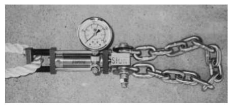
This thrustmeter was built by Cris Hawkins, and is set up for automated transducer recording of static thrust in addition to a direct gauge reading.
