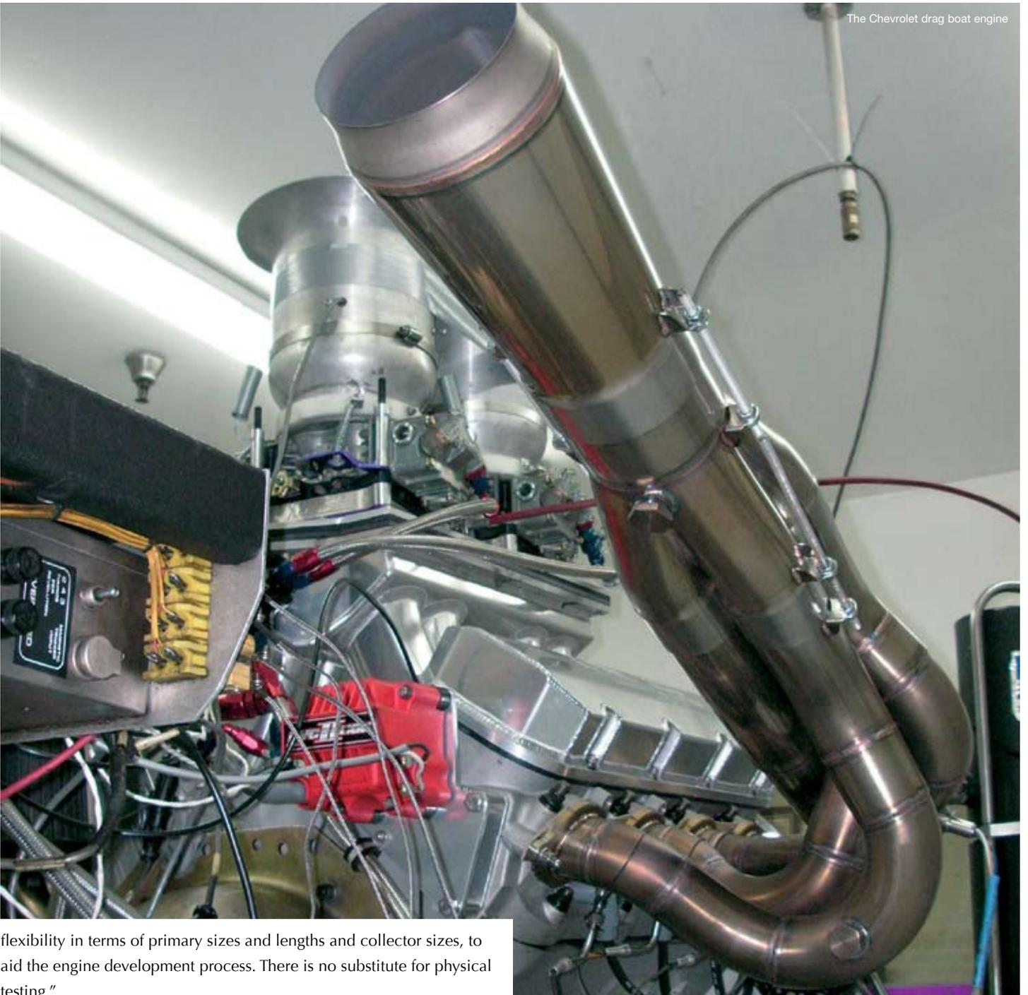
flexibility in terms of primary sizes and lengths and collector sizes, to aid the engine development process. There is no substitute for physical testing.”
