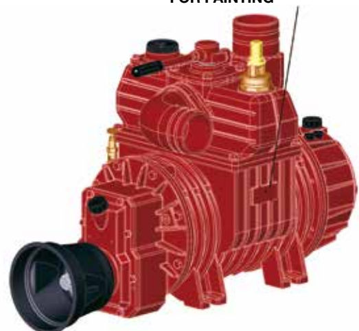
IDENTIFICATION LABEL WITH PROTECTIVE FILM FOR PAINTING
