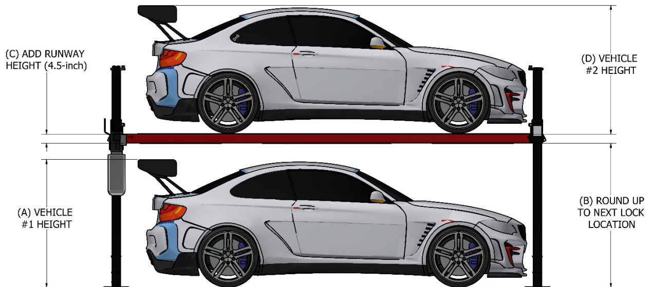
Figure 1.3 Lift Clearance (Height)
