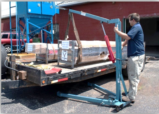
Figure 2.5: Material Handling Lift in Position
