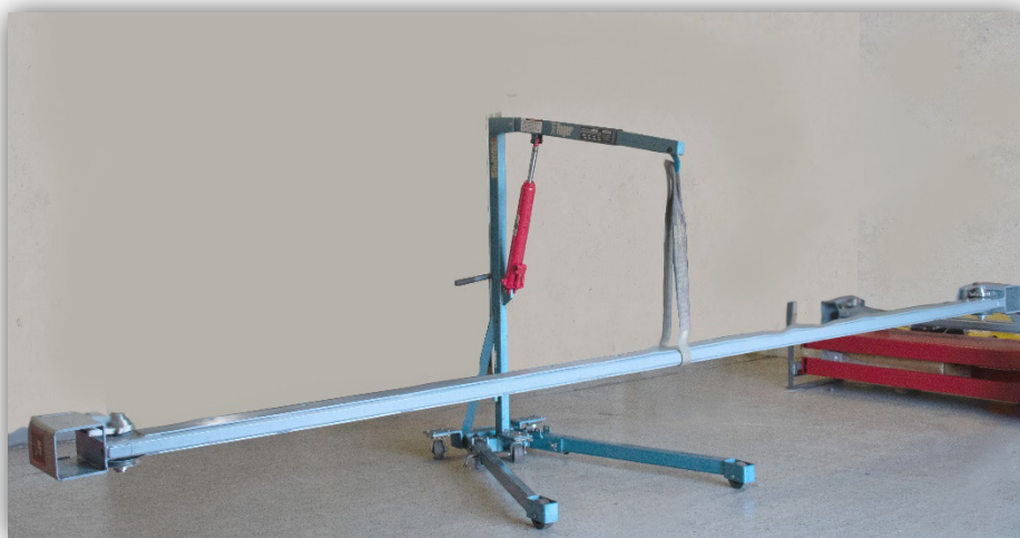
Figure 3.13 Moving the Crossmember
