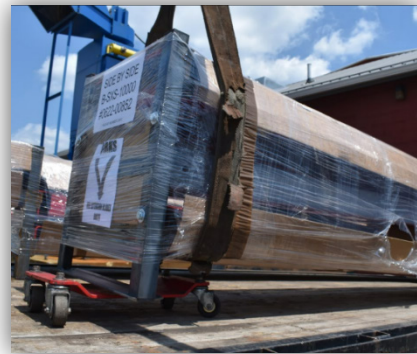
Figure 2.6: Positioning First Dolly
