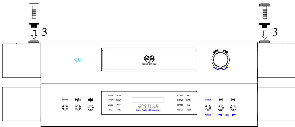
Figure 12 – Securing the Top Glass Plate
