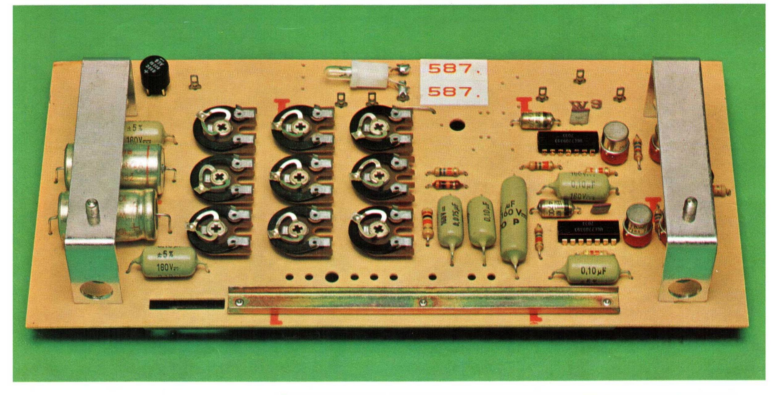
The introduction of a solid state control circuitry on the THORENS TD 125 Mk II transcription turntable has resulted in the complete elimination of the complex mechanical linkage associated with more conventional methods of speed control.
