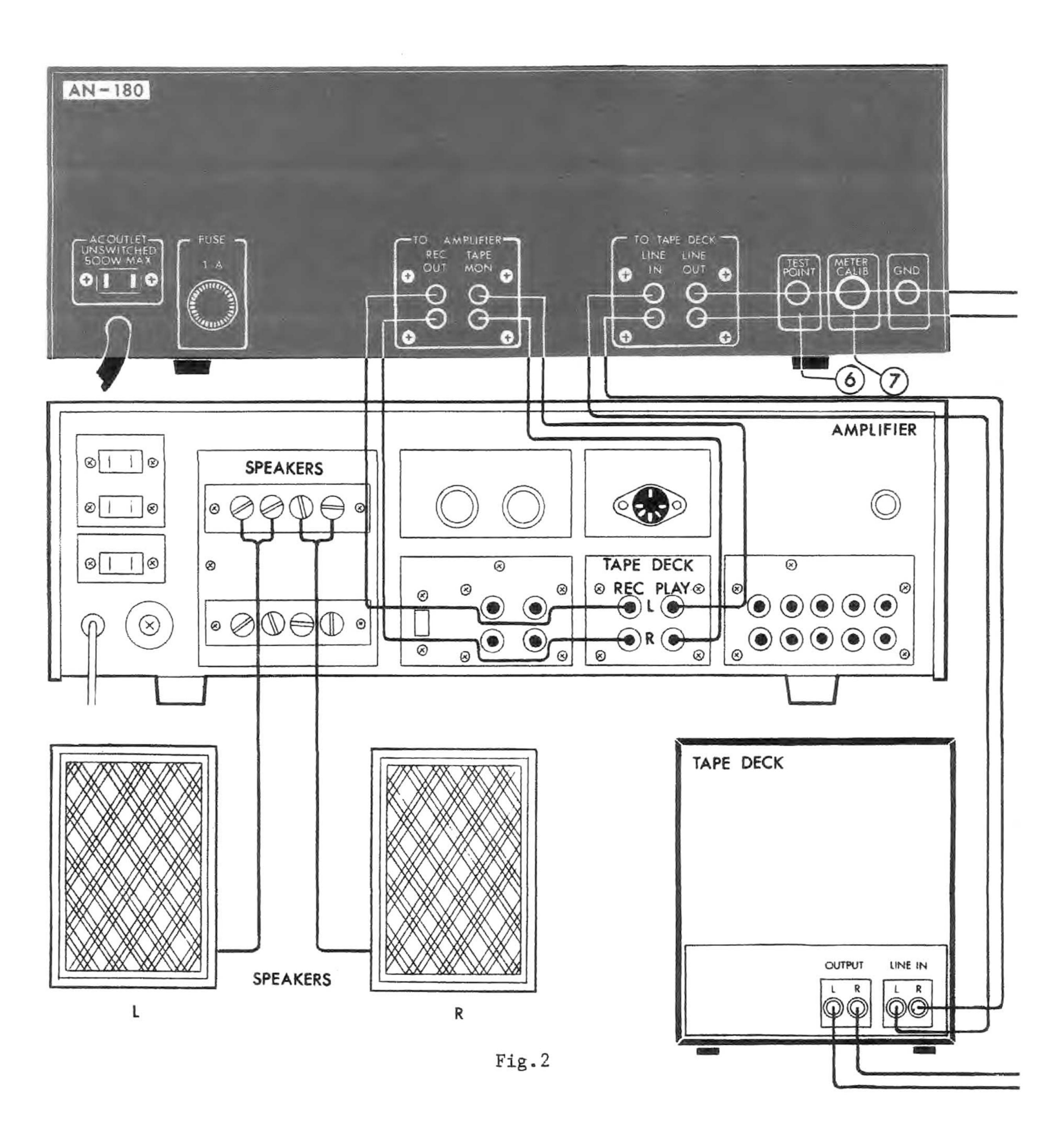
Connect cables to tape deck, Noise Reduction Unit and amplifier as shown in figure 2.
