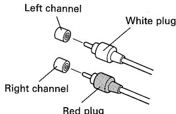
Connect the TAPE jacks of your amplifier to the LINE jacks of the cassette deck. Be sure to connect the REC (INPUT) jacks of the deck to the recording (output) jacks of the amplifier, and the PLAY (OUTPUT) jacks of the deck to the PLAY (INPUT) jacks of the amplifier.
