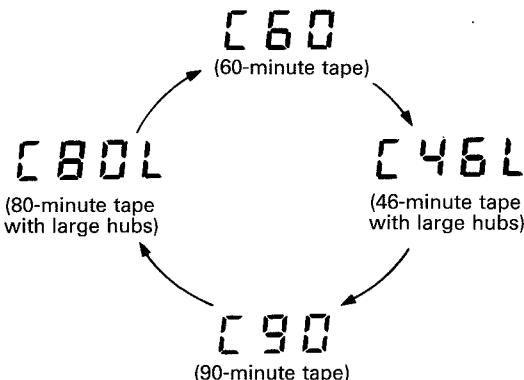
Set the tape capacity according to the length of the tape in use.
