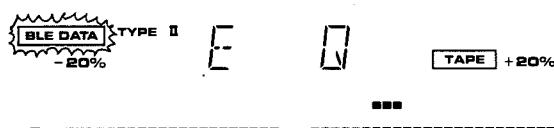
When the AUTO BLE tuning has been completed, the bias scale's standard position (the open segments) move to the same position as the upper setting position.
