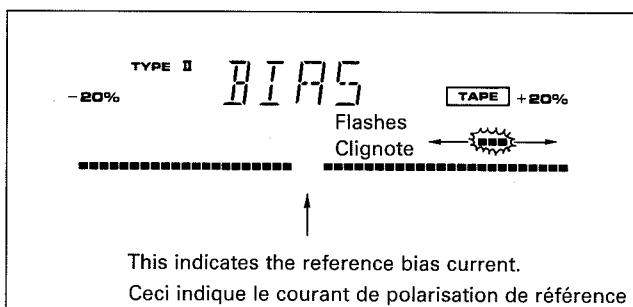
When the + or - BIAS button is pressed, the left and right channel level meters automatically change from bias mode to the previous mode after about 4 seconds.
