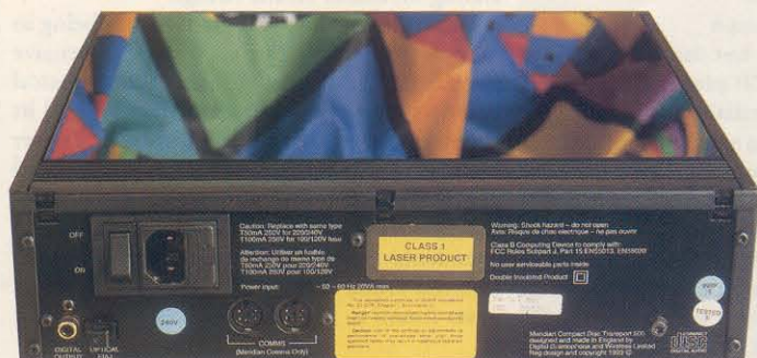
The 500 and 563 can be connected either by coax or optical leads
