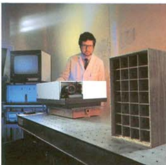
Electronic speckle pattern interferometry.
