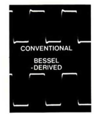
9 kHz square wave response shows complete absence of overshoot in the Bessel high filter design. Result: greatly reduced audible ringing and coloration.
