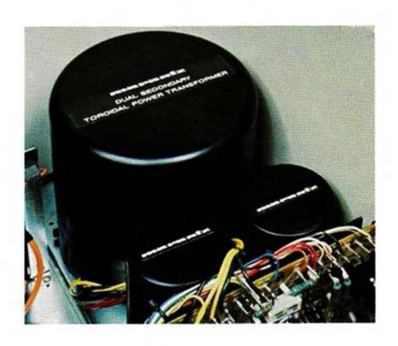
Complementing the transformer are high-capacity dual section electrolytic capacitors. This combination provides high power reserves, reliability and low distortion, while keeping heat and weight to a minimum.
