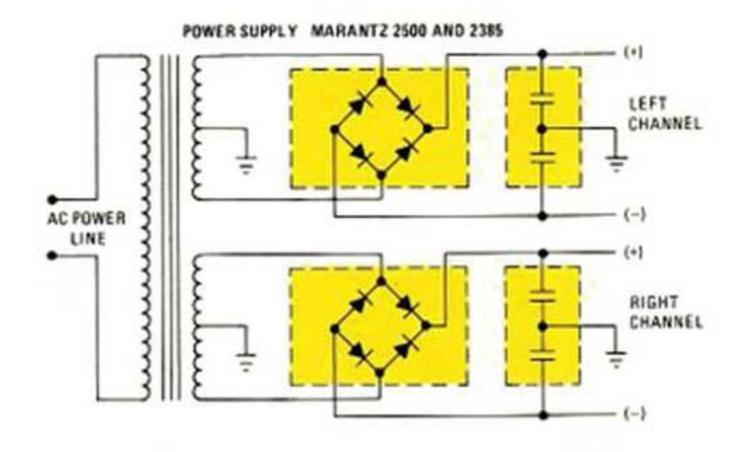
A specially designed toroidal-core power transformer with dual secondaries gives you two independent power supply sections. Each channel
