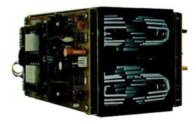
A built-in fan draws air through the tunnel and around the fins, creating turbulence that breaks up the insulating layer of warm air. The fan is thermostatically controlled to rotate slowly, quietly at low volume levels, and more rapidly at high volumes, when maximum airflow is needed.
