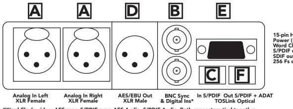
15-pin HD connector: Power (+12vdc) Word Clock out S/PDIF out SDIF out 256 Fs out
