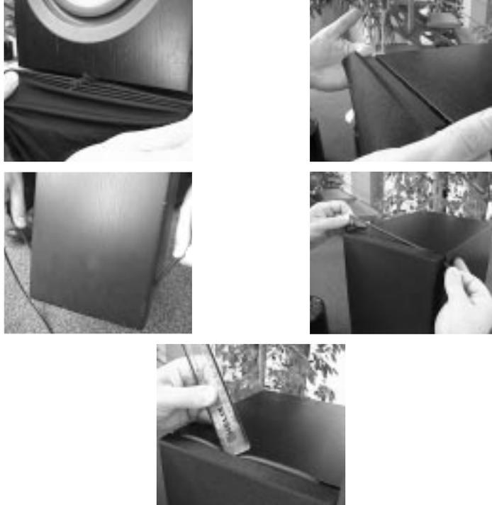
To remove the grille, grip the top right hand corner, pulling it so that the rubber ring and elastic clear the baffle. Then remove the ring and the grille cloth.
