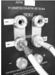
**BI-WIRING** Remove both linking plates. Leave the bottom two sockets unused.
