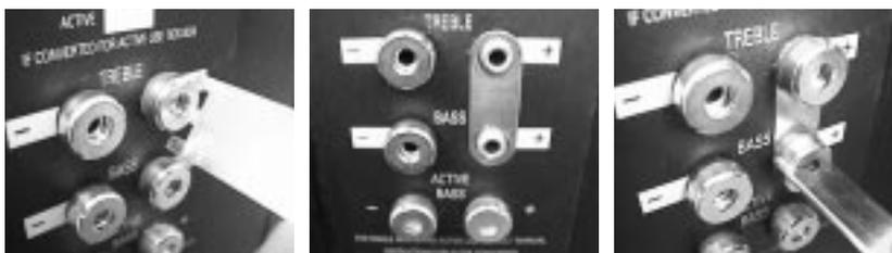
**IMPORTANT** Don't remove all the collars at once. Note that the lowest pair of sockets is only used in AKTIV mode. Don't connect to them at any other time.
