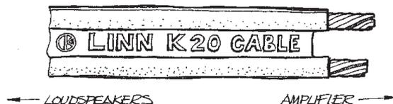
All Linn cable is marked with the Linn symbol to indicate directionality. The end marked with the circular Linn symbol should point to the loudspeakers, and the other to the amplifier.
