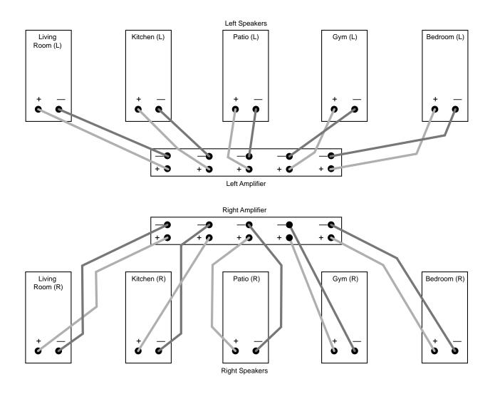
Another option is to use one amplifier to drive speakers in different rooms, using two channels to drive the left speakers and two channels to drive the right speakers. The diagram below illustrates this connection scenario:
