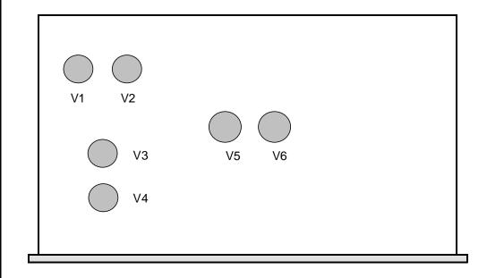
V1 AND V2 type 12AX7 V3 type 5751 V4 - V6 type 12AU7
