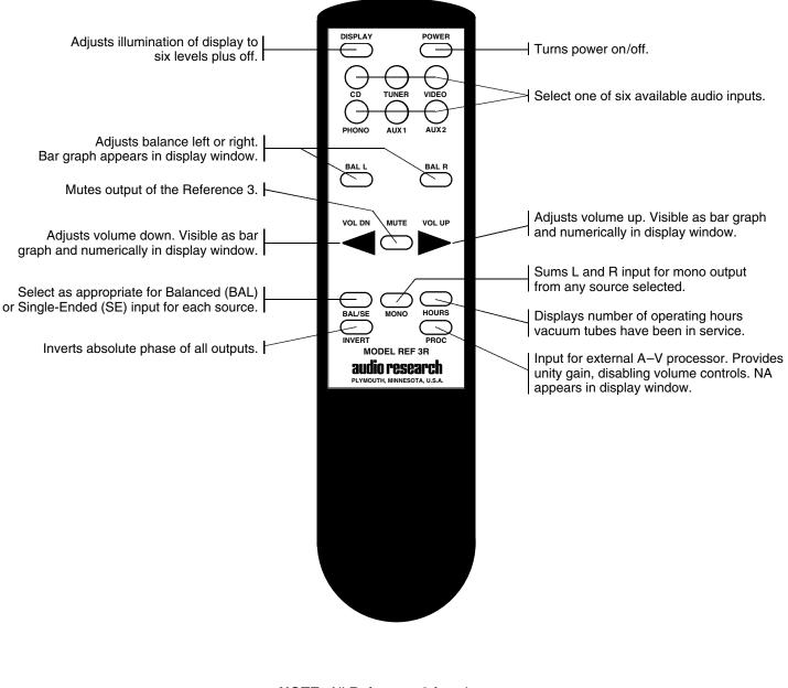
**NOTE:** All Reference 3 functions are available on the REF 3R hand held remote controller. All functions are indicated in the display window as they are selected. See "Description of Controls" in this manual for more information.
