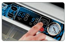
**Press to Vacuum Seal** Close lid, press the "Vacuum Seal" button and remove pouch from chamber when sealing process is complete.
