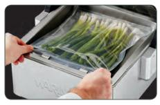
Place in Chamber Place filled pouch into chamber, position the open edge securely under pouch clips and flat across seal bar.
