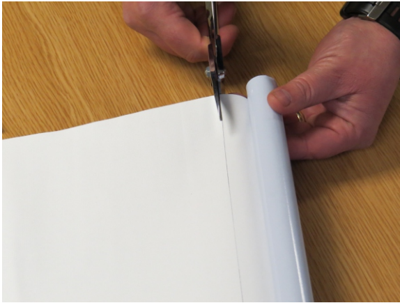
Step 5a. Cutting the blind - Option 1 Scissors
