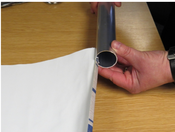
Step 10b. Fixing the fabric to the blind tube
