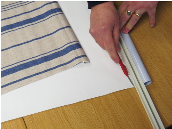
Step 5b. Cutting the blind - Option 2 Knife
