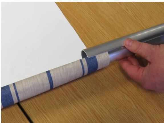
Step 10c. Fixing the fabric to the blind tube
