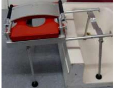
8. Using the adjustable non-skid swivel glides at the bottom of each leg, adjust the glides so that they raise or lower until the chair is stable within the tub, does not wobble or rock and provides for a level glide of the **seat assembly**. Loosen the hex nut on each of the glides first, then adjust the length of the bolts and finally re-tighten the hex nut to lock the length.
