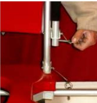
10. Remove the through-pins, securing the **armrests** in their folded position. Once the **armrests** are lowered, the through-pins may be inserted into, and through, the **armrests** and backrest supports, locking them in place. This will prevent the armrests from being raised.
