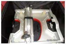
9. Repeat previous step with both of the leg assemblies on the **frame w/ tethered upper legs and Latch.**
