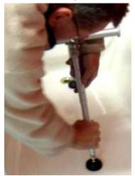
Note: The swivel feet have a 1+" adjustment range. Make big adjustments with the spring pins and fine adjustments with the swivel feet. ALWAYS CHECK THE SWIVEL FEET BEFORE USING THE CHAIR. Extending any too far out of its leg might cause it to be unstable or, even worse, to dislodge from the leg.
