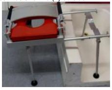
glides so that they raise or lower until the chair is stable within the tub, does not wobble or rock and provides for a level glide of the
