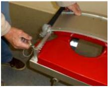
using the two through-pins. Ensure that the pins, when inserted through the diameter of the tubes, extend entirely through the tubes and lock firmly into place.
