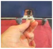
is slid either all the way across or back the retractable spring lock will engage automatically at the appropriate location.
