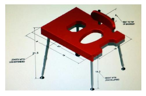
Weight-bearing capacity = 300 lbs maximum. Weight (in bag) = 19 lbs + 9 lbs (Transfer Accessory in bag) Bag Dims: Tub Chair: 7.5"x 20"x 11" / Transfer: 5.5"x 20"x 11"
