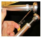
Note: The swivel feet have a 1+" adjustment range. Make big adjustments with the spring pins and fine adjustments with the swivel feet.
