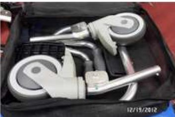
*are left and right caster legs.* Install them, ensuring that the colored dots on the lower legs match those on the upper legs (so the exposed bolt heads at the bend in each leg face outwardly from the chair).
