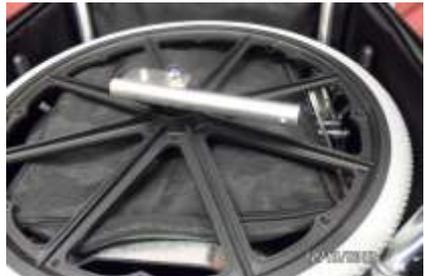
14. Place the remaining **20"-diameter wheel assembly** on top of the first one, this time, leg down such that the wheels are slightly offset from one another and the legs interlock.
