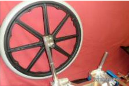
6. Install the first **20"-diameter wheel assembly** (removed from the case in step 1), by depressing the spring pin button on the leg extension of the **20"-diameter wheel assembly** and lowering the leg
