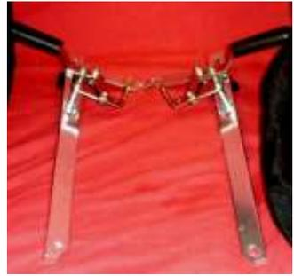
Install each **cross-brace w/ wheel lock** by placing its keyway over the protruding bolt head of its corresponding leg as indicated by the colored dots. Align the groove of both long and short sections, draw them together, pulling the wheel legs toward one another. Tighten the thumb screws to secure them.
