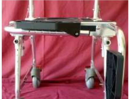
16. If mounting, or remounting, the seat cushion to the aluminum **seat assembly**, press the Velcro located on the front face of the cushion to the front of the chair first, then lower it on to Velcro located at the top of the aluminum seat pan, from front to back, as you stretch the cushion toward the rear of the seat.
