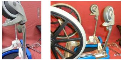
9. Remove the **rolling frame / seat assembly** from the travel case by grabbing the seat frame, turning it right-side-up and placing it on all four wheels.
