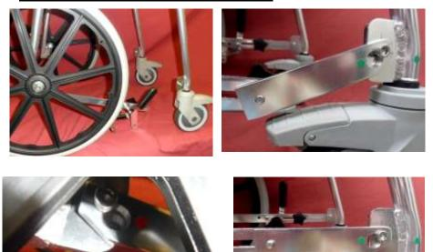
14. Remove the **push handles** from the **accessory pouch** and insert them into the openings located at the top of the backrest. Rotate them until the spring pin buttons pop into place through the holes provided.
