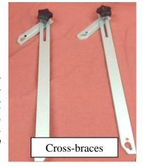
6. Remove both **cross-braces** from the zippered accessory bag. Loosen the black knobs allowing each **cross-brace** to unfold. There are left and right **cross-braces**. Install each **cross-brace** by placing its keyway over the protruding bolt head of its corresponding leg as indicated by the colored dots. Align the groove of both long and short sections and draw them together, pulling the front and rear **legs w/ swivel casters** toward one another. Tighten the black knobs to secure them.
