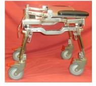
Using the spring pin buttons and adjustment holes in the telescoping legs, adjust the height of the **rolling frame** so that the occupant may safely and comfortably transfer to the "Go-Anywhere" Chair™. This may involve some trial and error. Ensure that the frame will fit over the commode as well, if necessary. Make sure that each telescoping leg is secure with a spring pin button protruding through one of the adjustment holes.
