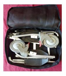
With the seat assembly still in the case, one-at-a-time, raise each of the (4) tethered upper legs (two have the lower legs w/ casters already installed) from the rolling frame, placing each into its corresponding leg socket, giving it a push until you feel it lock into place.
