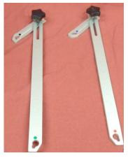
Remove the (2) cross-braces 6. from the zippered accessory bag. Loosen thumb screws allowing each cross-brace to unfold. There are left and right cross-braces. Install each cross-brace by placing its keyway over the protruding bolt head of its corresponding leg as indicated by the colored dots. Align the groove of both long and short sections, draw them together, pulling the caster legs toward one another. Tighten the thumb screws to secure them.
