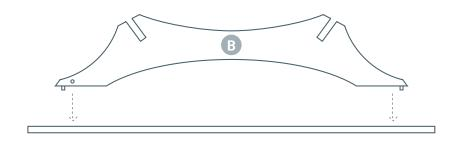
Slot leg pieces C and D into support (B) and align pins with slots in table top. Locate holes in C and D, insert allen wrech and rotate to lock. Turn over and enjoy!
