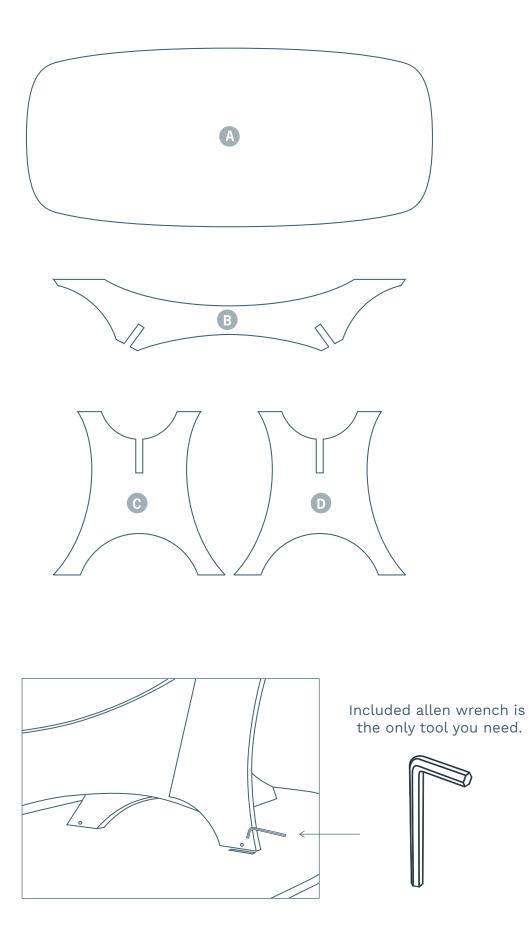
Attach leg support B to table top (A) by aligning dowels with holes in table top. Locate holes in B, insert allen wrech and rotate to lock.
