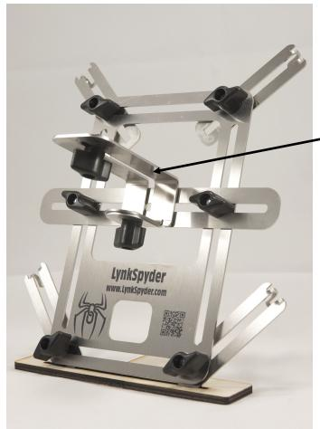
"Adapter Add-on" - (1) piece. This piece is used to allow for the use of traditional camcorders and small to medium cameras. It is advised that the "Spyder Slyder" be mounted with the tab on the bottom (as shown). Fasten the adapter to the Slyder using the included "Hex Bolt". It is recommended that you use a 7/16" wrench to firmly tighten the hex bolt in place.
