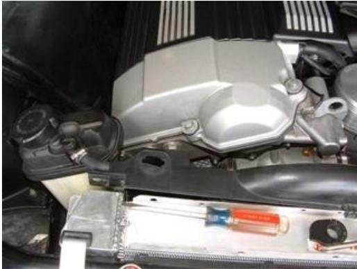
5. Remove the clutch fan using a thin 32mm wrench, turning the fan nut *clockwise*. If necessary, use a long screwdriver between two bolts on the water pump pulley to hold pulley while loosening the fan nut. Carefully work the fan up out of the fan shroud toward the right side of the radiator. Work one blade at a time around upper radiator hose.
