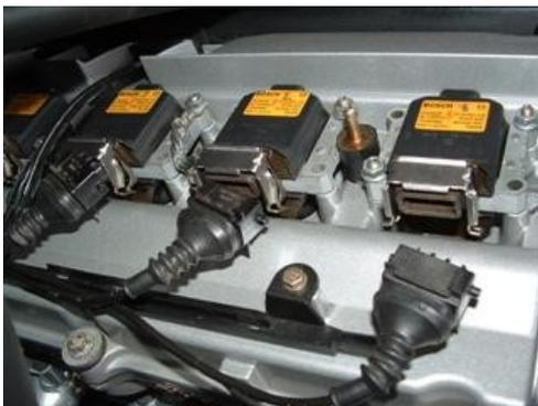
9. Carefully pull each coil wire from the hold down clips on the valve cover.
