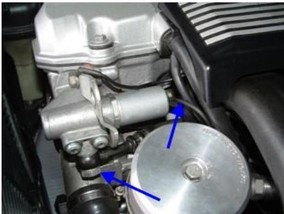
On OBD-I cars, remove the plastic cable cover that is attached at the bottom of the vanos. It is held on by two small e-clips. Be careful not to lose the e-clips!
