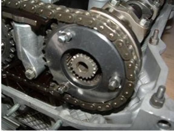
Now you should be able to slide the two cam gears and the timing chain off together. Replace chain if necessary.
