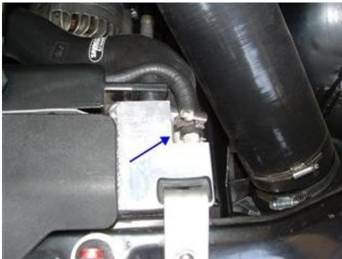
3. Now carefully remove the clip next to the radiator cap that sits around the bleed valve. It has two tabs that just need to be pushed towards each other and then lifted straight up. Leave the bleed screw tight.
