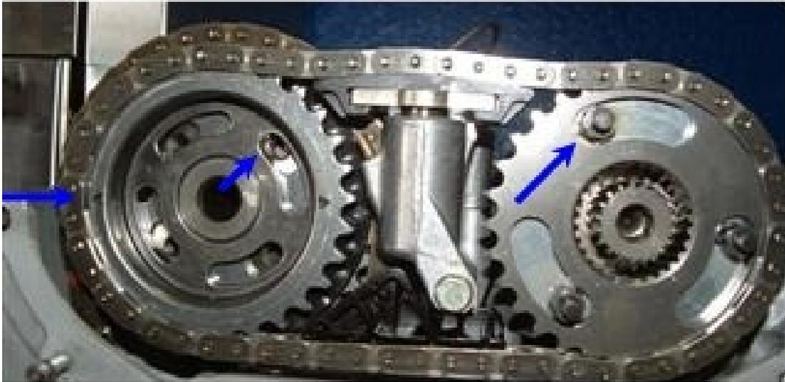
Install the washer on the exhaust cam gear, and then the 4 torx bolts. DO NOT fully tighten the torx bolts yet. Simply tighten them until they are snug then back them off a half turn.
