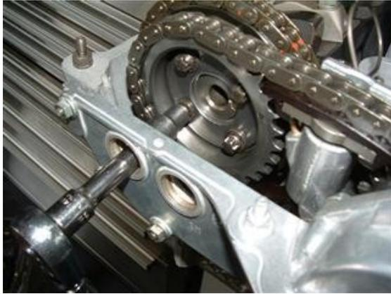
Now, use the sprocket turning tool on the exhaust cam gear and while rotating the tool clockwise, gently wiggle the vanos loose from the mounting studs and slide it out. This is easier with a second set of hands to wiggle the vanos loose while rotating the tool.
