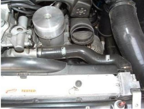
2. Carefully release pressure in the cooling system by *slowly* opening the coolant tank cap until all air has escaped, then re-tighten cap. On the driver's side of the radiator, loosen the hose clamp holding the small coolant return hose and pull hose off of the fitting. Remove the hose clamp and set it aside. Do NOT remove hose from coolant tank side.
