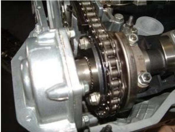
Now, while gently pushing against the vanos, slowly rotate the exhaust gear **counter-clockwise** until the intake gear catches the first available tooth on the cup. You shouldn't have to rotate the exhaust gear very far for the intake gear to catch. Once it catches, continue rotating the tool until the vanos is fully seated against the head.
