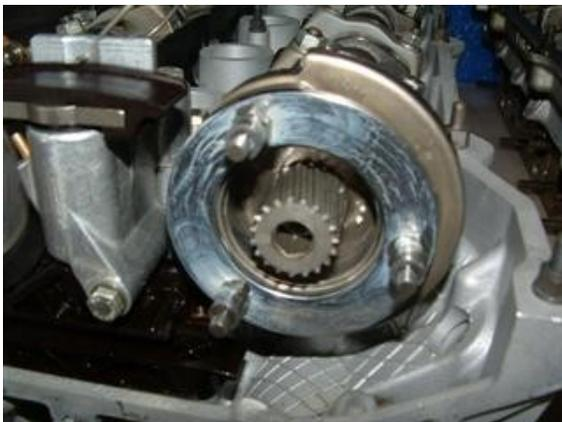
Reinstall the upper chain tensioner with the locking pin still in place.
