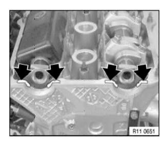
Check the valve cover gaskets. If they are brittle replace them. On OBD-1 cars, the gaskets sit on the head. On OBD-II cars, the gaskets sit in the valve cover.
