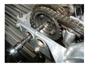
Now, use the sprocket turning tool on the exhaust cam gear and while rotating the tool clockwise, gently wiggle the vanos loose from the mounting studs and slide it out. This is easier with a second set of hands to wiggle the vanos loose while rotating the tool.
