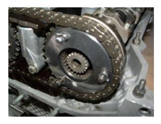
Now you should be able to slide the two cam gears and the timing chain off together. Replace chain if necessary.
