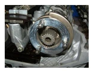
Reinstall the upper chain tensioner with the locking pin still in place.
