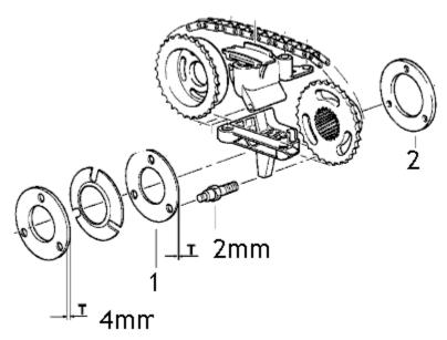
Remove the 3 mounting studs from the intake cam with a 10mm wrench. The cam block should hold the cam in place while loosening the studs.
