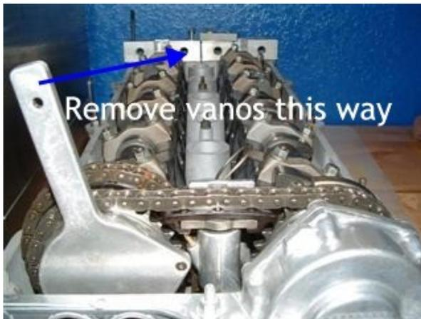
Remove any old RTV sealant from the head where the vanos was seated.
