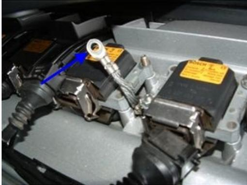
11. Now you can remove the bolts holding the valve cover down. There are 11 bolts around the perimeter and 4 in the middle. Two of the middle bolts will need the grounding straps removed first, (8mm nut) then the bolt itself can be removed. Note that these two have a stud on top for the grounding straps. Be sure to remove each washer and rubber gasket beneath each valve cover bolt before removing the valve cover so they don't get lost.
