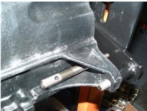
**Note:** Some aftermarket lightweight flywheels do not have the notch for the TDC pin. If you don't seem to have that notch, or are unable to get the pin into the block, do not fear. You will just have to use the small mirror and carefully align the timing marks the best that you can. As mentioned previously, removing the #1 spark plug and using a dial gauge can provide the most accurate results.
