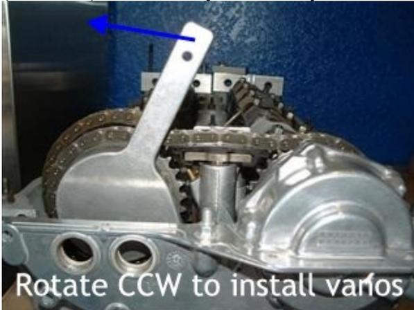
Once the vanos is fully seated, replace the six 10mm nuts, and the two 13mm bolts along with mounting bracket. Be sure the longer of the two 13mm bolts goes in the top hole, along with the ground wire (on OBD-I).
