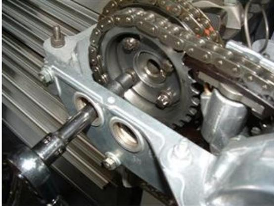
Now, use the sprocket turning tool on the exhaust cam gear and while rotating the tool clockwise, gently wiggle the vanos loose from the mounting studs and slide it out. This is easier with a second set of hands to wiggle the vanos loose while rotating the tool. Be careful because some oil will drain out of the vanos where you removed the banjo bolt!
