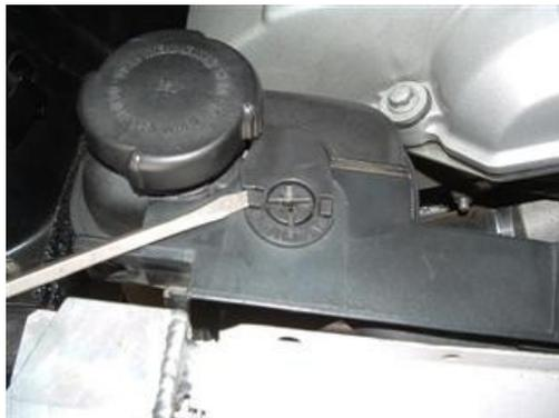
4. Move the expansion tank to the side by tilting it to the left. The top of the tank will slide under the fan shroud, pulling the detached return hose with it. Just move it far enough to gain clear access to the front of the vanos. Do not disconnect any other hoses!
