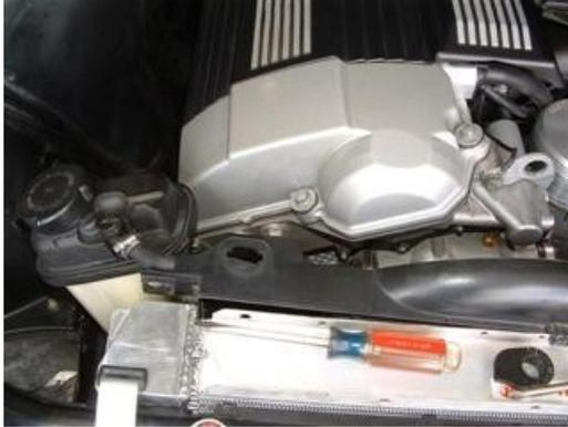
5. Remove the clutch fan using a thin 32mm wrench, turning the fan nut *clockwise*. If necessary, use a long screwdriver between two bolts on the water pump pulley to hold pulley while loosening the fan nut. Carefully work the fan up out of the fan shroud toward the right side of the radiator. Work one blade at a time around radiator hose.
