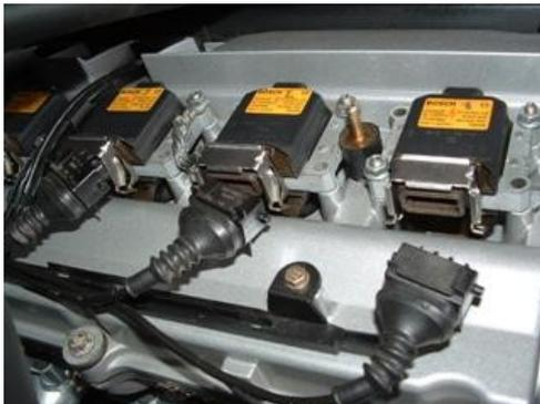
9. Carefully remove each coil wire from their hold down clips on the valve cover.
