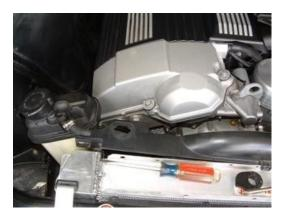
5. Remove the clutch fan using a thin 32mm wrench, turning the fan nut *clockwise*. If necessary, use a long screwdriver between two bolts on the water pump pulley to hold pulley while loosening the fan nut. Carefully work the fan up out of the fan shroud toward the right side of the radiator. Work one blade at a time around upper radiator hose.
