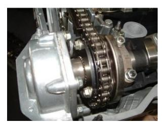
Now, while gently pushing against the vanos, slowly rotate the exhaust gear **counter**-clockwise until the intake gear catches the first available tooth on the cup. You shouldn't have to rotate the exhaust gear very far for the intake gear to catch. Once it catches, continue rotating the tool until the vanos is fully seated against the head.
