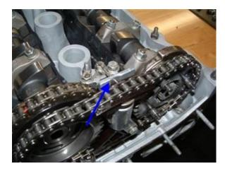
With the cam blocks still in place on the cams, loosen the 4 torx bolts on the exhaust cam gear about 1 full turn. DO NOT remove them! They just need to be loose enough to rotate the exhaust gear. You will use the two access holes in the vanos to reach the two lower torx bolts.
