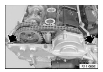
Apply a thin coat of RTV sealant at the corners of the half-moon transitions at the back of the cylinder head.
