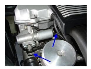
On OBD-I cars, remove the plastic cable cover that is attached at the bottom of the vanos. It is held on by two small e-clips. Be careful not to lose the e-clips!
