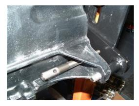
**Note:** Some aftermarket lightweight flywheels do not have the notch for the TDC pin. If you don't seem to have that notch, or are unable to get the pin into the block, do not fear. You will just have to use the small mirror and a carefully align the timing marks the best that you can. As mentioned previously, removing the #1 spark plug and using a dial gauge can provide the most accurate results.
