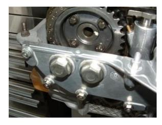
Remove the six 10mm nuts along the bottom of the vanos, and the two 13mm bolts that attach the engine hanger bracket to the front of the head/vanos. Remove the bracket.
