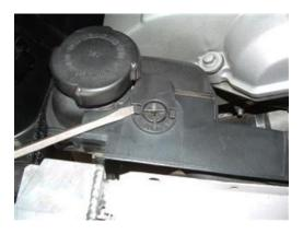
4. Move the expansion tank to the side by tilting it to the left. The top of the tank will slide under the fan shroud, pulling the detached return hose with it. Just move it far enough to gain clear access to the front of the vanos. Do not disconnect any other hoses!
