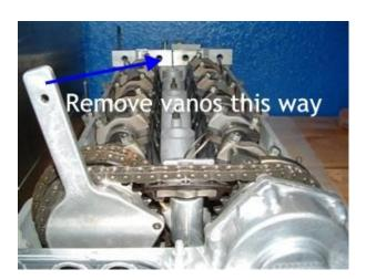
Remove any old RTV sealant from the head where the vanos was seated.
