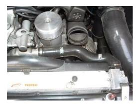
2. Carefully release pressure in the cooling system by *slowly* opening the coolant tank cap until all air has escaped, then re-tighten cap. On the driver's side of the radiator, loosen the hose clamp holding the small coolant return hose and pull hose off of the fitting. Remove the hose clamp and set it aside. Do NOT remove hose from coolant tank side.
