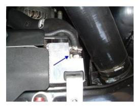
3. Now carefully remove the clip next to the radiator cap that sits around the bleed valve. It has two tabs that just need to be pushed towards each other and then lifted straight up. Leave the bleed screw tight.
