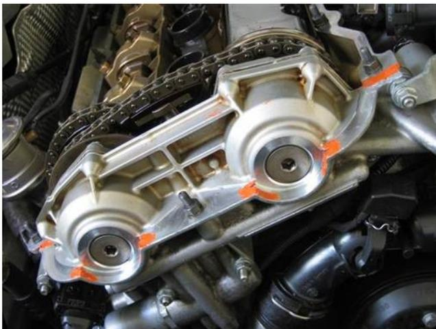
Place a thin coat of RTV sealant at 2 engine vanos/head contact points, and at vanos/head front and rear half moon corners. Allow sealant to set for ~2 minutes before installing valve cover.
