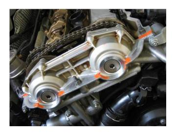
Place a thin coat of RTV sealant at 2 engine vanos/head contact points, and at vanos/head front <u>and rear</u> half moon corners. Allow sealant to set for ~2 minutes before installing valve cover. Reinstall valve cover, coil packs, and related parts.
