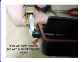
**#19** Now you can remove the pin with a small pair of diagonal cutters.
