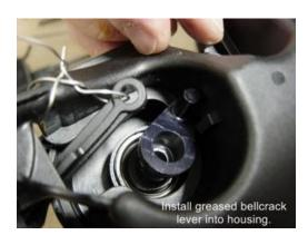
Note the rotational alignment of the bell crank lever as shown and insert the new lubed up lever into the DISA housing. Push the lever all the way in.
