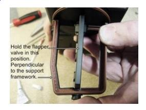
You will need to position the flapper valve properly before pushing the bell crank lever into place. This is the position you want the flapper valve to be in, 90 degrees (perpendicular) to the support framework. You will need to hold the flapper valve in this position for the next step.
