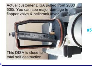
The last thing to check before installing the kit is the frame and bearing boss. On rare occasions when there is extreme wear like what's shown in the picture, the flapper valve can come completely loose from the part of the mechanism that controls its movement. If this happens the flapper valve can bend back and forth inside the intake manifold and damage or crack the upper bearing support. Clean around the area shown in the next picture and check for any signs of cracking.
