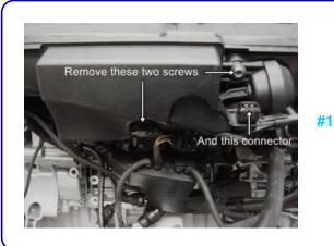
Start by removing the old DISA unit from the intake manifold by removing the two T40 Torx screws and one electrical connector securing the DISA. SLOWLY pull the DISA from the manifold. There is a steel pin in the end of the DISA housing (shown partially removed in the next picture) that can come loose and fall into the manifold during removal. Make sure that the pin is still in place on your DISA after removal. If not, Do not start the engine again until the pin is located.
