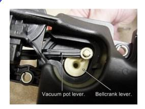
This is what's under the cover. The creme colored piece is the bell crank lever which rotates the flapper valve. This is the piece that typically wears out and causes most of the problems. The black piece is the lever that connects the vacuum pot diaphragm to the bell crank lever.
