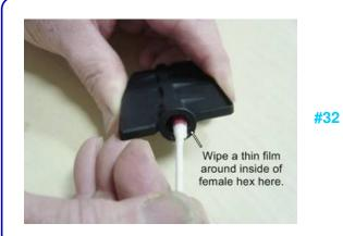
Now wipe a thin film inside the female hex pocket of the new flapper valve. Don't over do it, it should just be wet on the sides. You don't want excess that will wick into the bearing during assembly. Note: The next 9 steps, up through step # 41, need to be performed within about 5 minutes of applying the threadlock in this step. 5 minutes is plenty of time so there is no need to rush.
