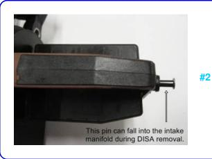
Make sure that this pin is still in the DISA after removal. If not, it has probably fallen into the intake manifold as you removed the DISA. If the pin has fallen into the manifold it should be able to be easily retrieved through the DISA opening in the manifold. DO NOT proceed until you locate this pin.
