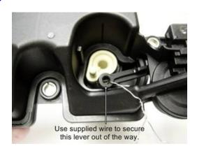
Using the supplied safety wire, secure the vacuum lever off to the side to keep it out of the way. This is not a necessary step but is very helpful.
