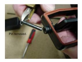
Here is the steel pin removed. It's pressed in pretty tightly on a new unit. This is what has ruined a few engines after it fell out and went through the intake runner and into the combustion chamber.
