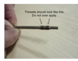
Anything more than this is unnecessary. Excess theadlock could try to make it's way into the end bearing so don't feel the need to over do it.
