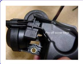
The installation begins by removing the actuator access cover. You'll need a small flat blade screwdriver. Push in and pry up at the location shown. The cover pops off easily.
