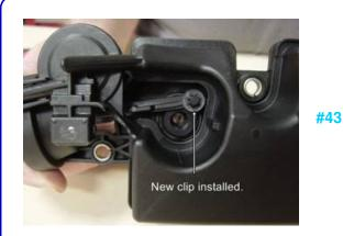
Double check that the flapper valve can be rotated to the closed position and back open without binding. If you manually close the valve, then release it, the valve should spring back to the fully open position, except as noted below.
