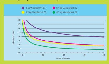
Modern production facilities need the flexibility to change raw material or to run with mixtures, for example wheat with rye. The figure shows the unique properties of Viscoferm® at a mash containing 50% wheat and 50% rye.
