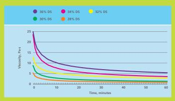
Viscoferm® effectively reduces the viscosity of mashes with high dry substance, making it a unique enzyme product for High Gravity Fermentation (HGF). With a dosage of 0.3 kg Viscoferm/t DS the viscosity of mashes with 100% dry-milled rye can be reduced by 80%. By using Viscoferm, rye mash slurries with as high as 36% DS can be made pumpable and easy to process. Viscoferm enables similar viscosity reduction for mashes of wheat, barley, and triticale.
