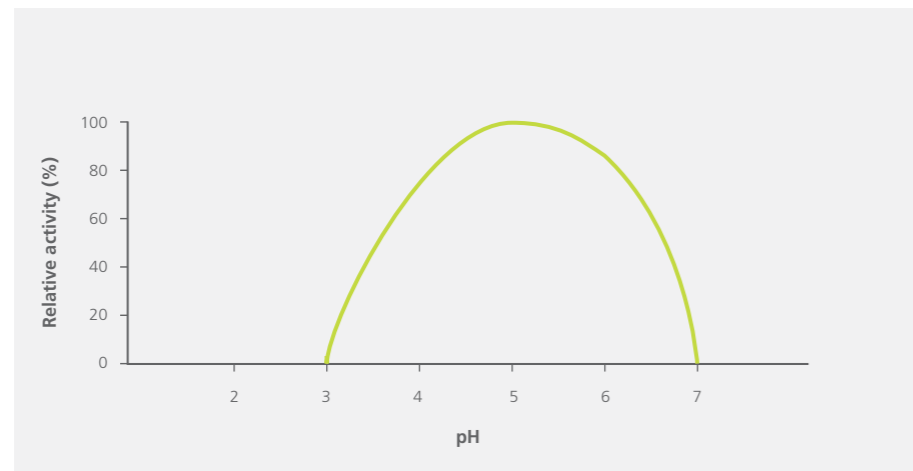
Fig. 5.4-4 B. pH dependency of Novozymes Finizym® 250 L
