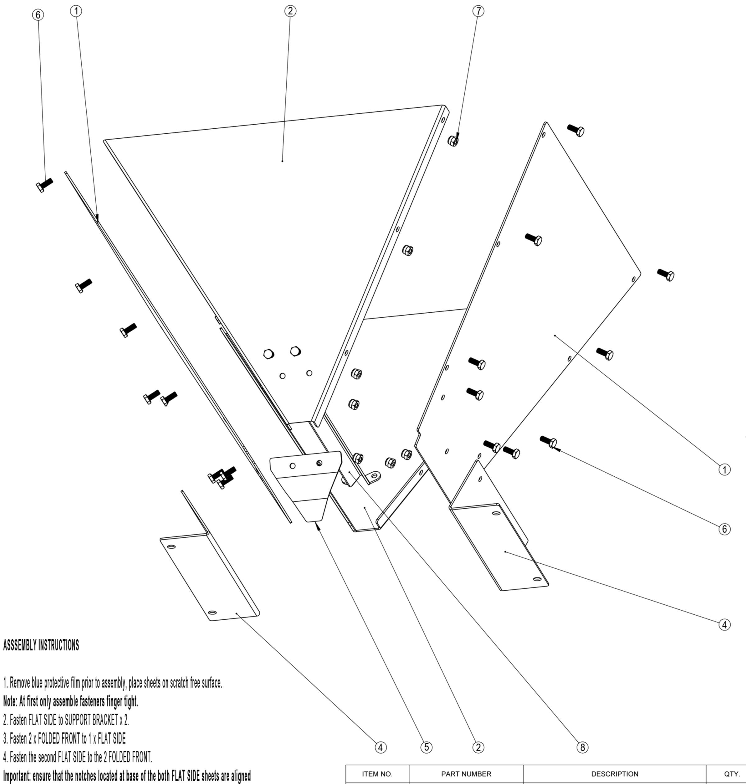
5. Assemble GEAR GUARD FEEDER and the GEAR GUARD inside the hopper.
