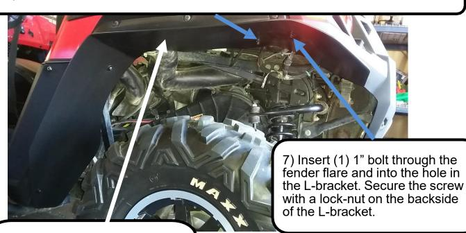
Add self-tapping screws in the upper portion of the fender if you have any gaps after you tighten all of the hard ware.
