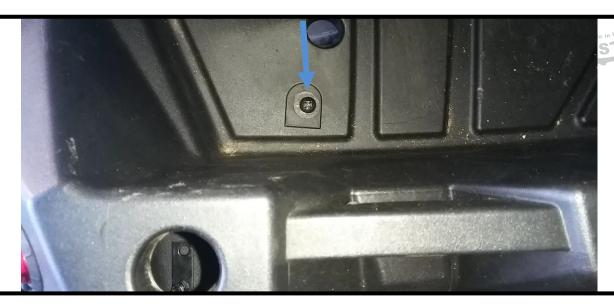
6) With the 2" bolt installed, press the fender against the threaded end of the bolt, add a washer, and a lock-nut.
