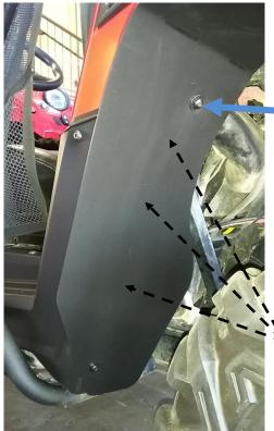
4) Proceed to the next hole located near the bend in the factor fender. Insert (1) 1" bolt and (1) washer through the bottom of the fender and through the hole. Add (1) washer and (1) lock nut on the exposed thread on the back side, but do not tighten the nut yet.\*
