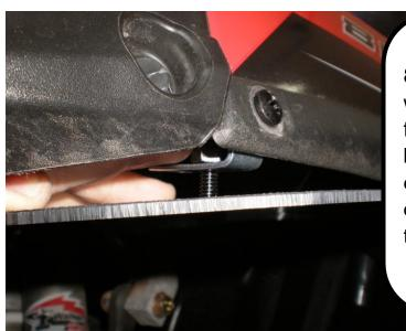
8) Insert (1) 1/4" X 3/4" bolt and (1) washer through the bottom of the fender and through the front 1.5" L-bracket. Thread (1) lock nut on the exposed thread and tighten the bolt. All of the remaining hardware can be tightened at this point.
