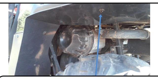
5) Have a friend hold the bend of the fender extension tight against the angle in the factory fender. Insert (1) 1/4" X 3/4" Phillips bolt and (1) washer through the bottom of the fender and the forward 2" L-bracket. Thread (1) lock nut on the exposed thread and tighten the bolt as your friend holds the fender tight against the bend. Repeat this step with the last remaining hole and 1.5" L-bracket.
