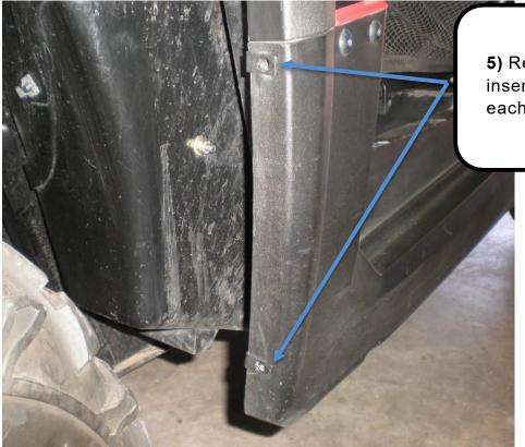
**5)** Remove the inner plastic rivets and insert (1) U-Nut on the inside edge of each hole.
