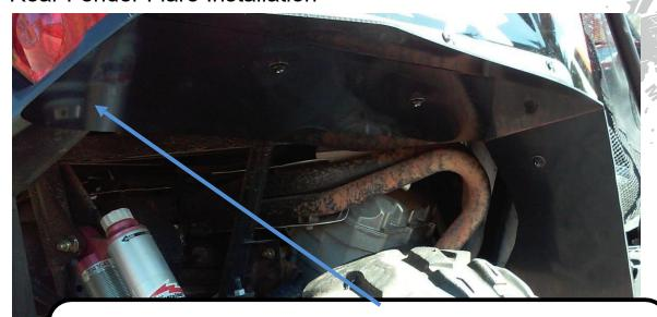
Note: Self-tapping screws can be installed to reduce any remaining gaps after all of the aforementioned hardware has been tightened down. The L-Brackets can also be bent or manipulated to reduce gaps as well.
