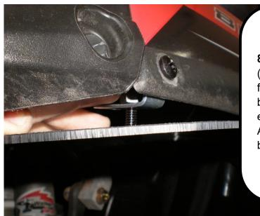
8) Insert (1) 1/4" X 3/4" Phillips bolt and (1) washer through the bottom of the fender and through the front 1.5" L-bracket. Thread (1) lock nut on the exposed thread and tighten the bolt. All of the remaining hardware can be tightened at this point.
