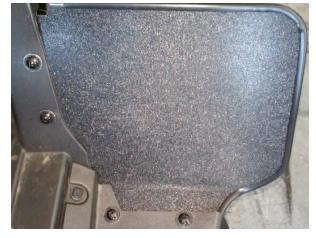
3) Complete the installation of the rear fenders by re-installing the "No-Step" frame protector. Insert the front clip between the tube and the fender flare as pictured below. It's a tight fit, but it will slip right in. Once the front section is in place, push the rear portion of the plastic down so you can re-insert the plastic rivet.
