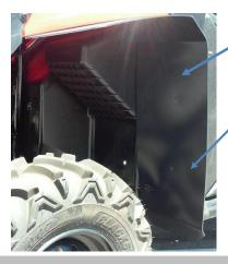
\*The fender Lbrackets (fender hangers) may need to be bent slightly for proper fitment of the fenders.
