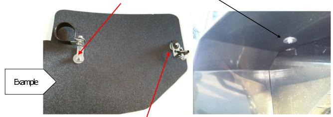
5) Insert (1) 1/4" x 3/4" Phillips bolt with a washer into the hole located toward the front of the fender flare. Reach around the top of the fender and slide a washer between the spring clamp on the hanger and the fender. Tighten down the bolt using a screwdriver.
