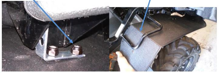
6) At this point, the fender flare should be hanging from the L-bracket you just installed. Remember, the lock-nuts securing the L-bracket to the fender flare should not be tight.
