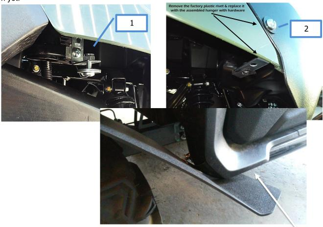
3) Install the front fender flares by inserting a roll bar clamp around the lower tube chassis while adding (1) 1/4"x 3/4" Phillips bolt, (2) washers on both sides, and a lock nut on the back side (but do not tighten it down yet). Adjust the fender so that it's nicely tucked into the top corner of the factory fender. Once the roll-bar clamp and hangers line up with the holes in the fender flare, the fender flare hardware can be tightened down (see below). You may find it necessary
