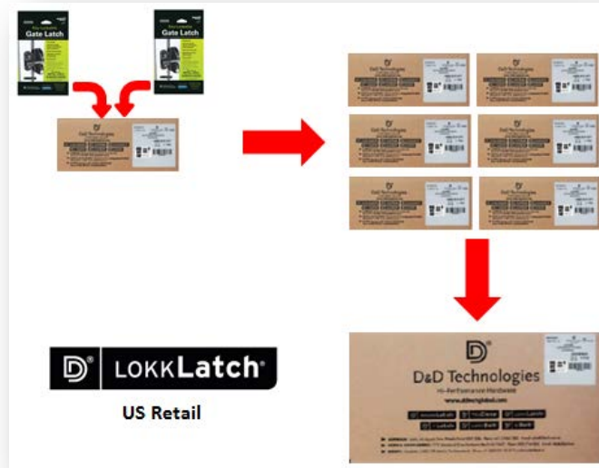
Figure 5.3. Current 2*6 inner and outer carton packaging configuration for our US Retail Product (LLAARS).
