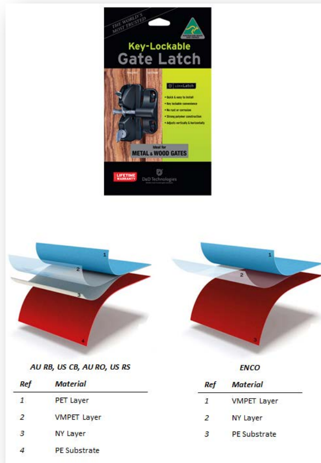
Figure 5.5. Illustration of the laminate structure for the Retail Product Line).
