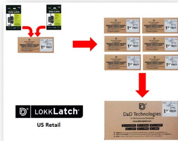
Figure 5.1. Previous 2*6 inner and outer carton packaging configuration for our US Retail Product (LLAARS).
