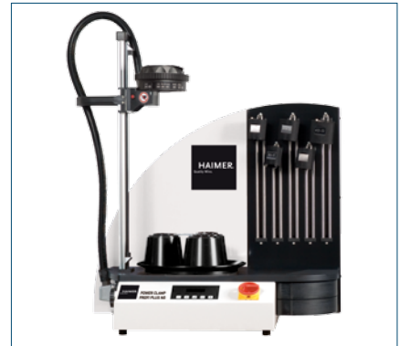
Power Clamp Profi Plus NG High powered shrink fit machine – Heating power 20 kW – For shrinking of tools from \varnothing 1/8"–2" (3–50 mm) – For HSS- and solid carbide tools – Big coil for \varnothing 1 1/2"–2" (40–50 mm) optional – Incl. rotary table and chuck support – Incl. tool tray – With craning boxes for accessories
