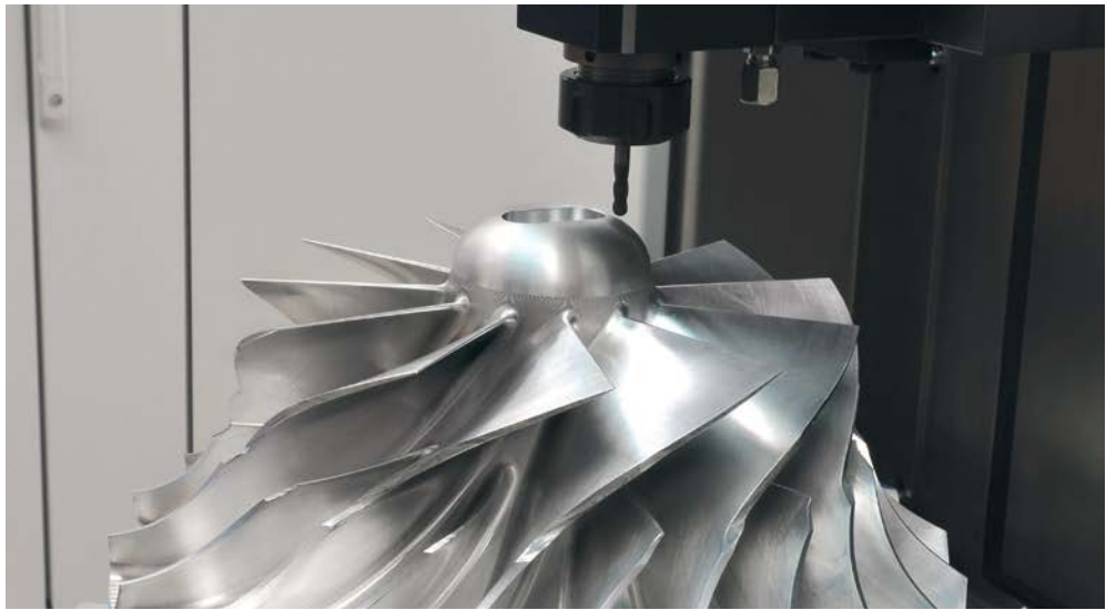
Compressor wheel for turbocharger Balancing by peripheral milling axial.
