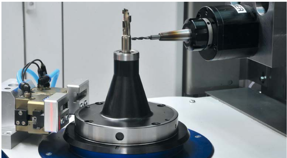
Balancing of tools with a HG balancing adapter for tools with a cylindrical shank For further information please go to p. 42.
