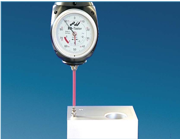
Measure surface flatness
