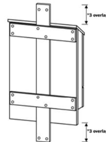
5) Pre-drill holes at the top and bottom of the vertical mounting boards, and secure the bat houses to the post with lag screws, hex bolts, or carriage bolts.
